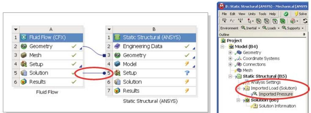
Drag-and-drop multiphysics: forming a link in the project schematic (at left) achieves data transfer between the different physics, and creates imported loads in the downstream simulation (shown inside the ANSYS Mechanical application at right).
