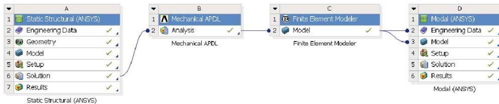
Chain systems together to achieve creative solutions to real-world engineering problems. Shown above is a static structural analysis that was performed to determine the deformation of a structure in response to applied loads. An ANSYS Parametric Design Language (APDL) script was used to export the mesh for the deformed shape to FE Modeler. FE Modeler was used to synthesize a geometry that was then used to perform modal analysis of the deformed shape.
