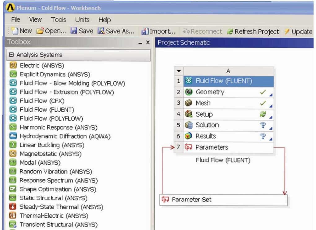
After dragging the desired analysis system into the project schematic, work through the system from top to bottom to complete your analysis. Icons in the right of each cell clearly indicate progress. Here the analysis is complete through meshing.
