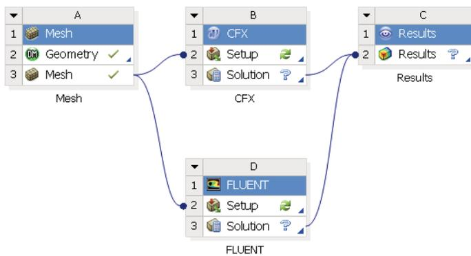
Here component systems have been used to represent a specific intent. A common mesh is used for analyses in ANSYS CFX and ANSYS FLUENT products, and the results are compared in the ANSYS CFD-Post tool using the Results system at right.
