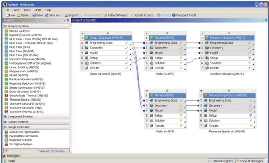
The new project schematic view shows an overall view of the entire simulation project. Engineering intent, data relationships and the state of the entire project are visible at a glance, even for complex analyses involving multiple physics.
